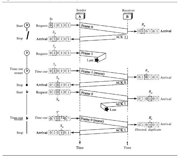
Figure 11.11 Flow diagram for Example 11.3
