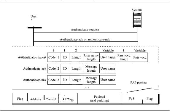
Figure 11.36 PAP packets encapsulated in a PPP frame
