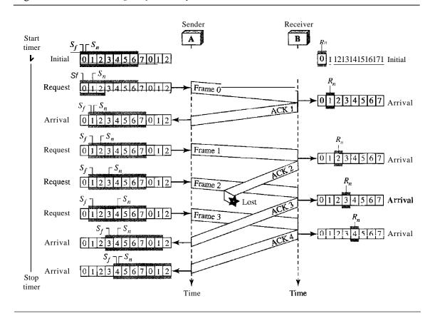
Figure 11.16 Flow diagram for Example 11.6
