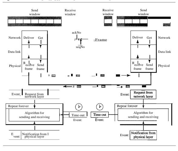
Figure 11.24 Design ofpiggybacking in Go-Back-NARQ
