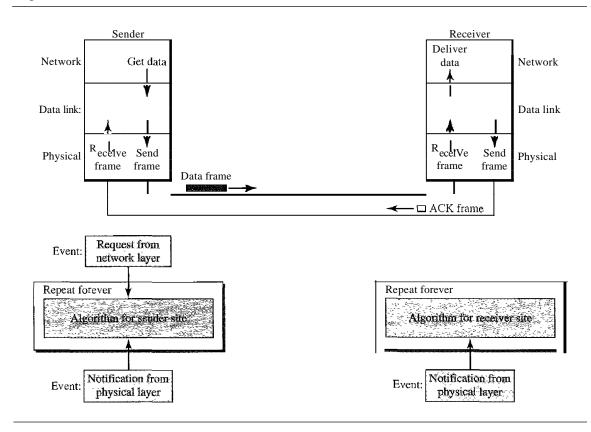
Figure 11.8 Design of Stop-and-Wait Protocol
