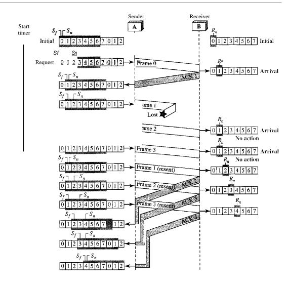
Figure 11.17 Flow diagram for Example 11.7
